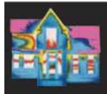
Without insulation, valuable energy escapes through the sides of your home.
