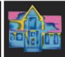
With insulation, pathways for energy loss are sealed off to prevent energy loss year-round.
